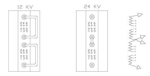
Figure 16 – Tapping regulation with double voltage
