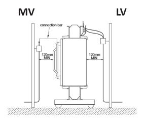
Figure 14 - Cables coming from the bottom.
