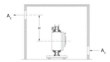
The minimum size of the openings to guarantee sufficient airflow inside the installation room (considering average annual temperature of 20°C) can be calculated using the following formulae:
