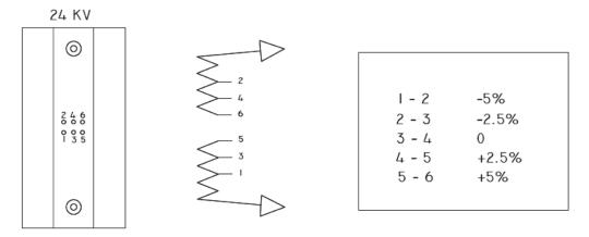
Figure 15 – Tapping regulation with single voltage
