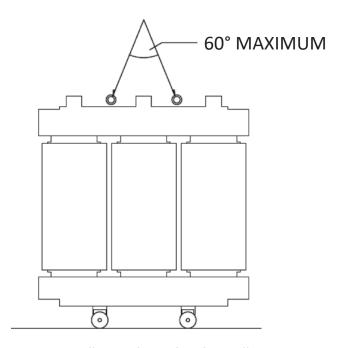
Figure 4 – Handling with overhead-travelling crane
